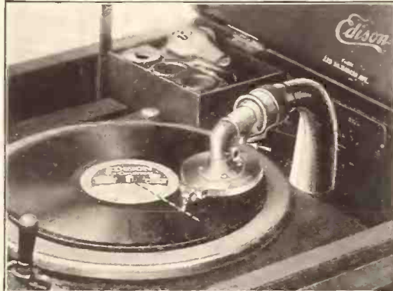
Illustrating position for playing Edison or other vertical cut records. Fibre, jewel or diamond point may be used as desired.
