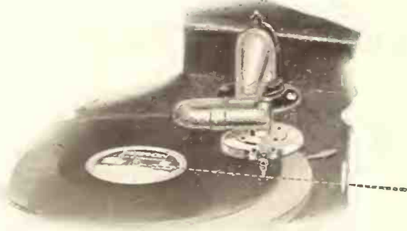
Showing position for playing Edison records—Fibre needle shown in reproducer.
