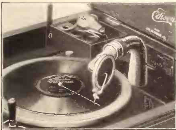
Illustrating position for playing Victor or all lateral cut records on the Edison phonograph.
