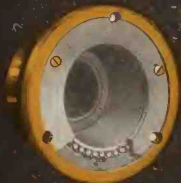
BALL BEARING No obstruction in the base
