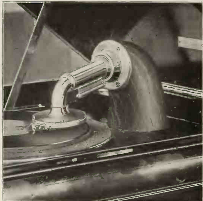
Reproducer in position for playing vertical cut records. Correct position for playing EDISON records.
