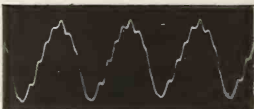
VIOLIN—The tone of the violin has many partial tones. None of these are aggressively dominant, however, hence the fluent, smooth quality of the instrument. This is shown in the photograph of its tone wave.
