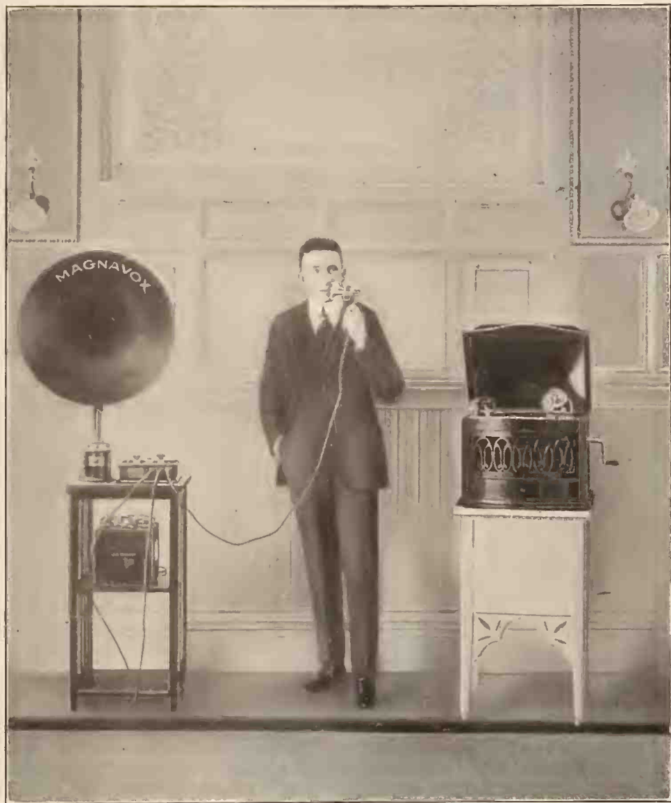
Fig. 1—Complete Equipment Showing Hand Transmitter in Use for Amplifying Voice
