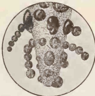
No. 2.—About one twenty-fifth of an inch of the point of a talking machine needle, greatly magnified. The rust has assumed the form of beads.
