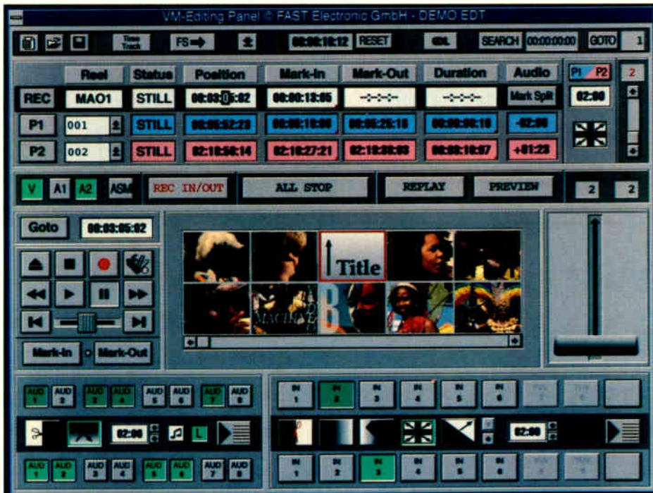
The Fast Video Machine can be used as an off-line hard disk recorder or an on-line editor.
