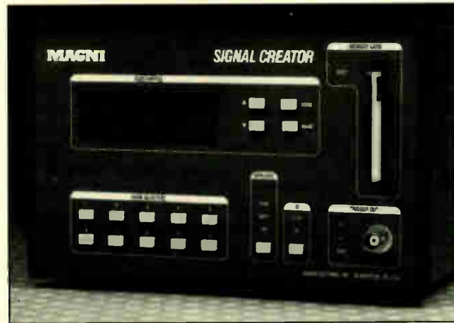
The Magni Signal Creator has dual video standard capability.
