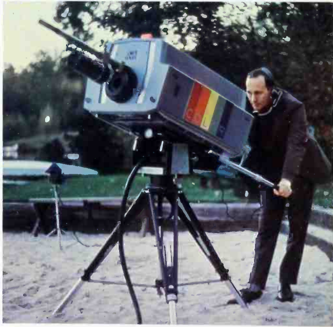
RCA Color Camera set up to test technical capabilities. A casegrain type telescope, focal length 125 inches, was installed on the Camera to produce the moon-shot shown here.
