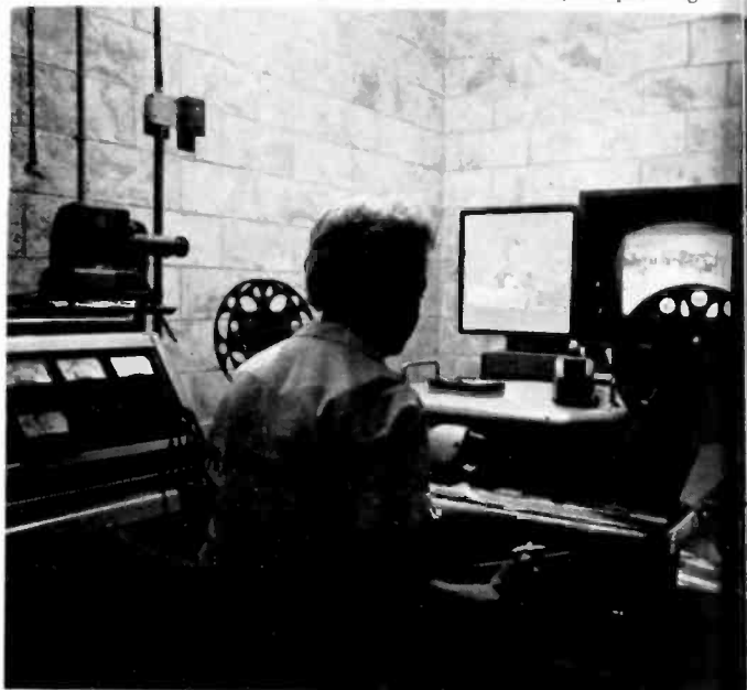
A timer electronically adjusts negative's colors before printing
