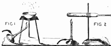
Fig. 1 shows a beautiful experiment with ammonium bichromate; on simple heating it deflagrates brilliantly. Fig. 2 shows the preparation of pyrophoric lead by heating lead tartrate in a sealed glass tube.
