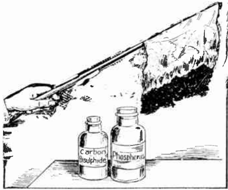
A paper flag is dipped into a solution of phosphorus in carbon bisulphide, held in the air and perhaps waved about a little, is soon ignited and burns with a slow flame.
