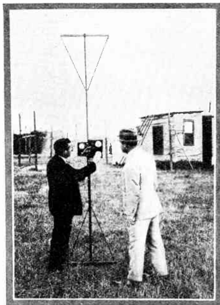
Of great importance were the field measurements on the strength of the radiated energy in the vicinity of the transmitter. Note compact and portable equipment.
