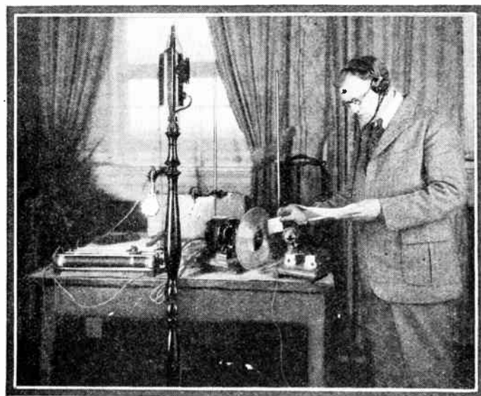
Dr. Wold, in front of the microphone at W G Y, broadcasting "The Voice of the Electron." A rotating, perforated disc through which a stream of light is allowed to pass operates a photo-electric cell which converts the light energy into electronic energy and results in the production of musical notes.
