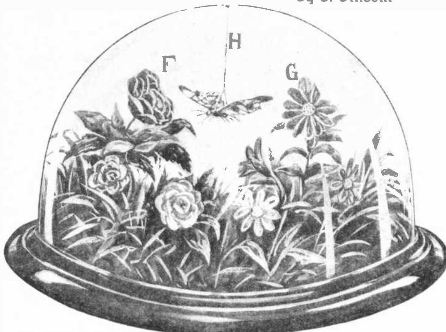
Fig. 4. A butterfly swinging by a slender thread from the top of a glass globe keeps swinging back and forth from flower F to flower G and back again for years. The mystery lies in a concealed voltaic pile. The butterfly has a metallic surface which touches a metallized surface on the flowers, each flower being connected to a terminal of the battery.
