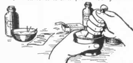
Mixing the semi-liquid solutions in a mortar with which the ends of safety matches are to be coated. Do not pulverize the mixture except when moist.
