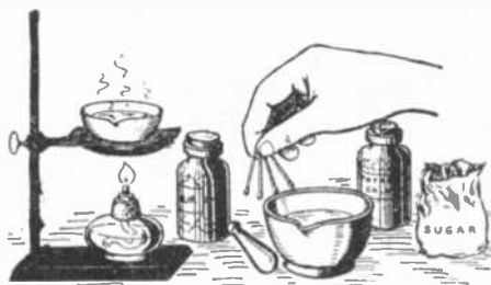
Making reproductions of the first match; a mixture of sulphur, potassium chlorate and sugar constituting the head is ignited by being touched to fuming sulphuric acid absorbed in asbestos. By no means pulverize the sugar and potassium chlorate together, or you may have an explosion.
