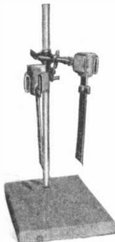
A glass support for electrodes; the rod is taken from a towel rack. The use of glass for the supporting rod ensures good insulation of the electrodes.
