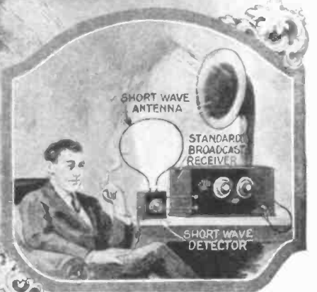
A radio receiver of the future employing a short wave pick-up device that feeds into a receiving set similar to those in use today. Note that a very small single turn loop aerial is sufficient to receive the short waves.
