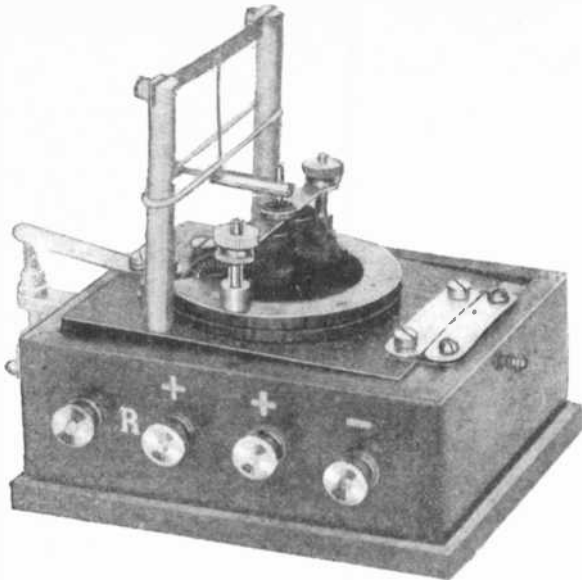
The Tauleigne amplifier opened up. Contact pressure between carbon point and button is varied by screw at left that tips it
