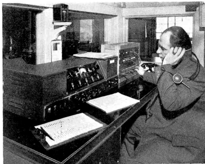
HAROLD HUGHES, Control and recording engineer at console thru which all WWVA programs pass regardless of whether they originate at the network in New York or from our studios. This is the heart of the Station.
