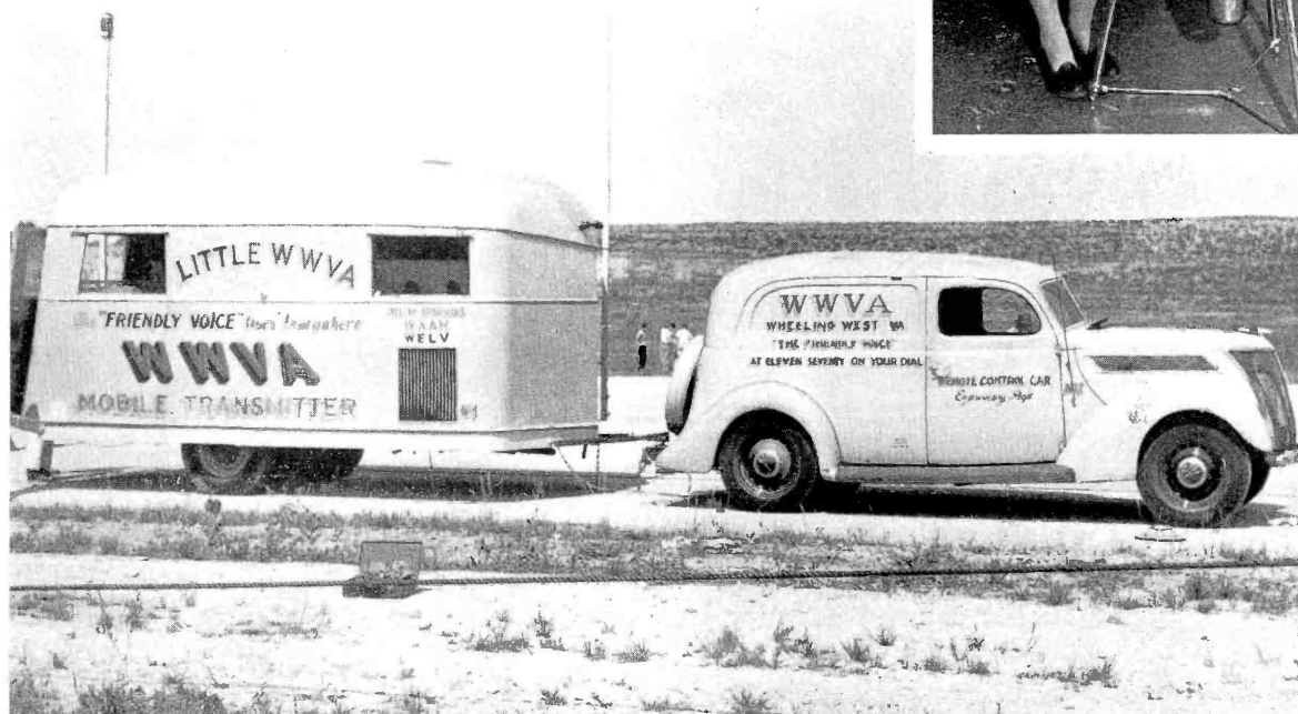
"LITTLE WWVA" carries two short-wave transmitters which permit programs to originate anywhere and be sent by short-wave to the main studios for re-broadcasting. A gasoline driven generator provides power for all operation.
