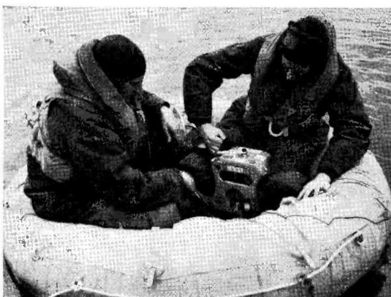
Two fliers, adrift in an RCAF rescue dinghy, operate a "coffee grinder" radio transmitter which can send out an SOS signal for 150 miles. The antenna for the "coffee grinder" is pulled aloft by a balloon. (RCAF photo)
