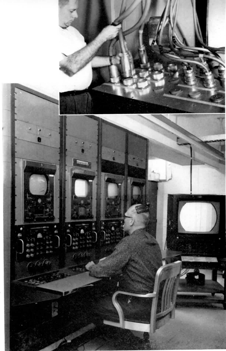
FIG. 16. The four live studio color cameras are controlled here. ▶
