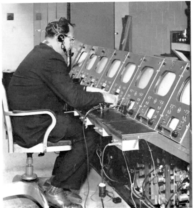
FIG. 19. Eight TK-11 cameras are adjusted from this position in master control.
