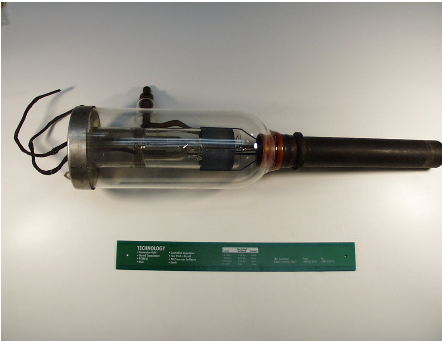
Transmitter Power tubes circa 1925, the improved-design second largest glass RF power tubes with large anode(plate) contact outside for water cooling system which can dissipate more power
