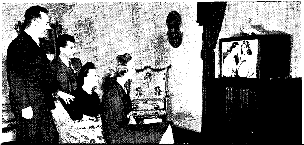
EXPERIMENTAL MODEL OF PROJECTION-TYPE HOME TELEVISION RECEIVER, DEVELOPED BY RCA, PRESENTS A CLEAR 18 BY 24-INCH PICTURE IN MOTION.
