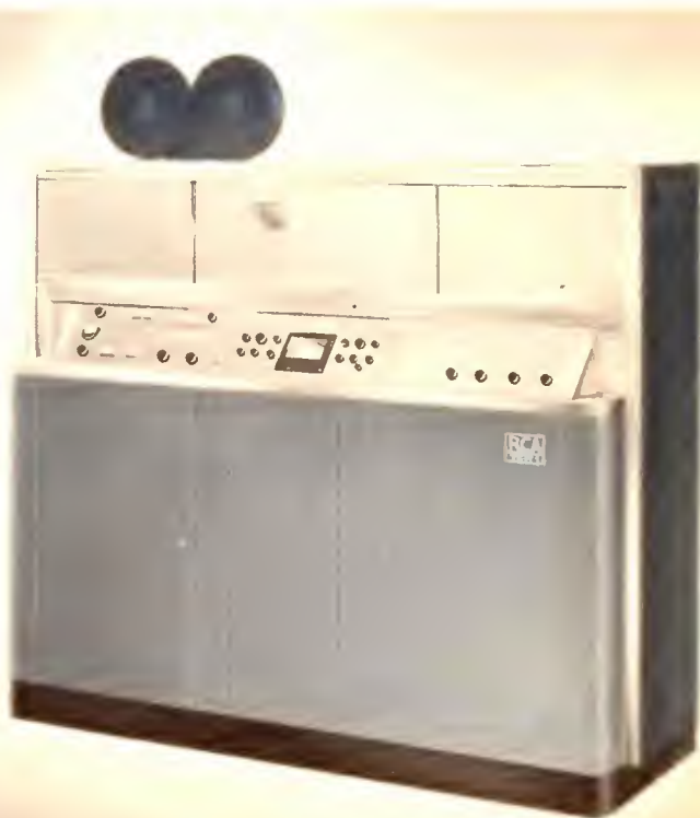
TFR-1 TELEVISION FILM RECORDER. New high-resolution Kine eliminates face plate distortions, resolves up to 900 lines, provides highlight brightness of 160-foot lamberts. New double-aperture camera eliminates shutter bar, lessens vibration. Self-compensating circuits assure uniform contrast, automatic control of exposure. Used with fast film developer to play back pictures in 2 minutes.
