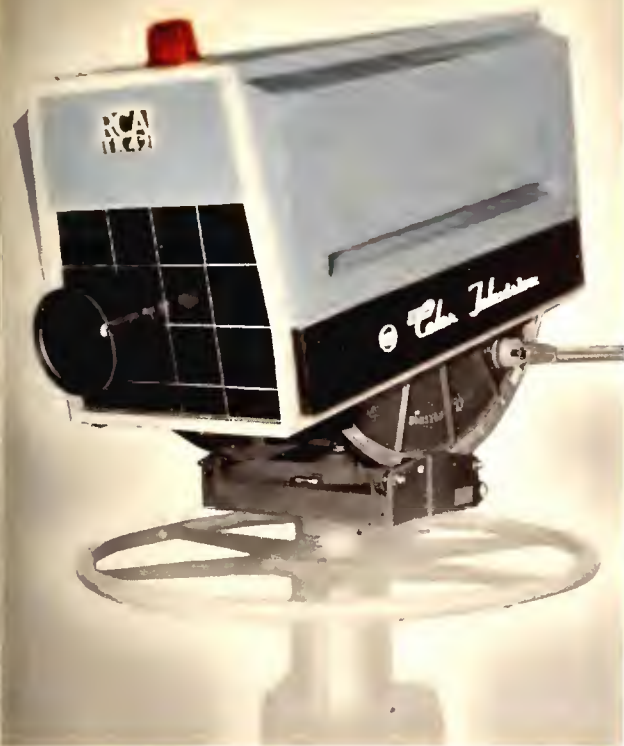
TK-42X COLOR CAMERA. New "M-Channel" design adds a monochrome channel to the red, blue and green color channels. As in four-color printing, the black improves color detail, and reduces registration problems. Also provides a striking "black and white from color" picture.
