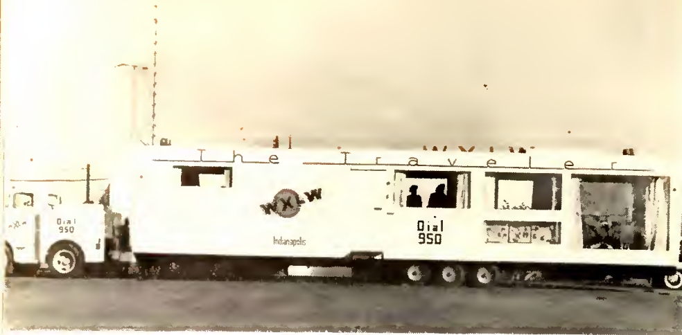
THE TRAVELLER , self-sustaining Mobile studio and transmitter of WXLW, Indianapolis, is contained in a 45-foot trailer unit. Towing unit generator can produce 10,000 watts of power
