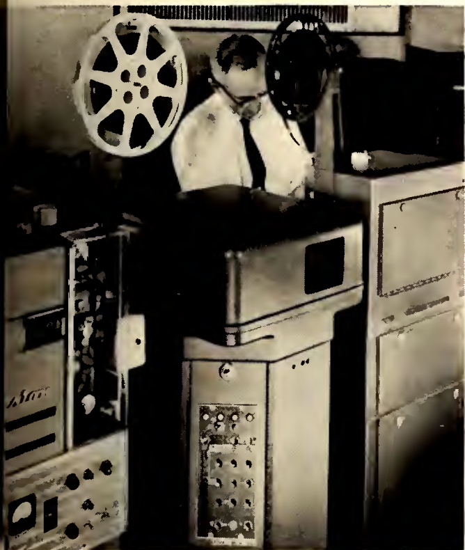
PROTECTION SYSTEM. RCA TP-6 16 mm professional projectors are used to double-up with 35 mm network projectors to insure on-air continuity in event of mishap. TP-6's are used throughout ABC local film rooms.
