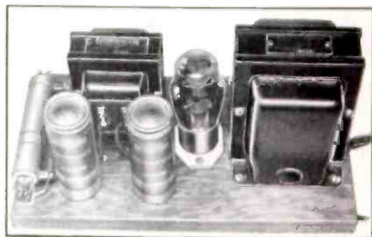
The 400-volt power-supply used with the oscillator.
