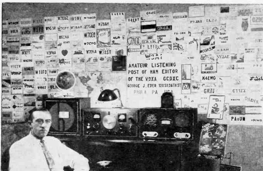
GEORGE J. EDER, 128 So. 36th St., Philadelphia is "HAM" Editor of WDXA and GCDXC, member Radex Club, and of the Short Wave League. His layout comprises a 20 meter 1/2 wave doublet, an RSR-Clipper Receiver, an SX-16 receiver, and a 12 PM Hallicrafter's Speaker. On phone, he has heard 103 Countries, of which 50 are verified. Forty-five states are also verified on 20 m. fone, out of 48 heard. He has been DXing on the broadcast band since 1920, the Amateur band since 1935, and QSLing Ham stations since 1937. He has 230 cards, and wants to QSL all states of U. S. and all countries heard on 20 meter fone, all states on 10 meter and 75 meter phone.
