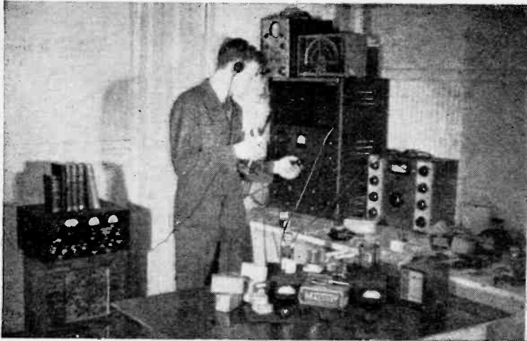
Picture at left shows test laboratory where the R. & T. "pull-swing" F-M system has been developed. Below—close-up of the parts used in building the amplifier here described. A high frequency amplifier, to operate efficiently on 59.2 mc., requires carefully selected parts. The Hallicrafter S27 receiver used in checking the R. & T. "pull-swing" apparatus is shown at the extreme left.
