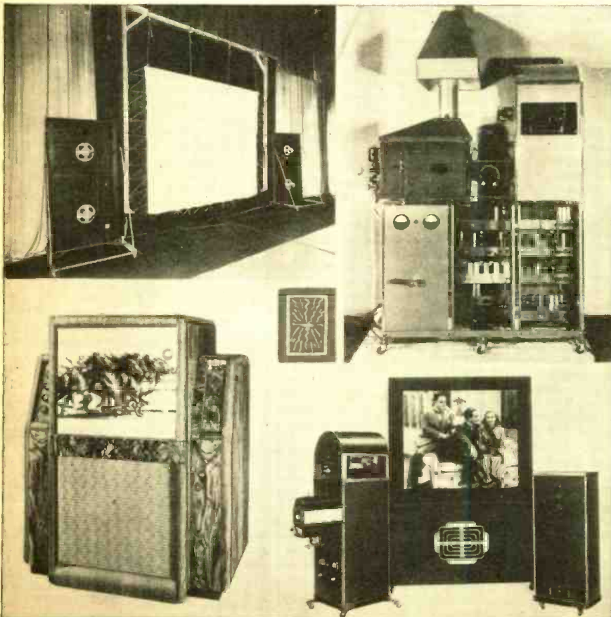
Two top pictures (below) show Scophony large image television screen, with loudspeakers on either side, and mirror drum projection scanner used in reproducing these images. Two lower photos show Scophony "home-model" television receiver, and a larger size receiver intended for public halls, stores, etc.
