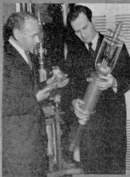
Right—Tubes for Television. Gilbert Seldes (left), television program director, and Dr. Peter Goldmark, chief television engineer, inspect the largest and smallest water-cooled tubes used in the new CBS television transmitter. The large power tube has 15,000 watts peak output and is three feet long. Below—In the new CBS television transmitter, this transformer, one of ten, weighs 5215 pounds and is cooled by 212 pounds of oil. 120 gallons of water per minute are needed to cool other parts of the transmitter, a complete air conditioning unit cools the water.
