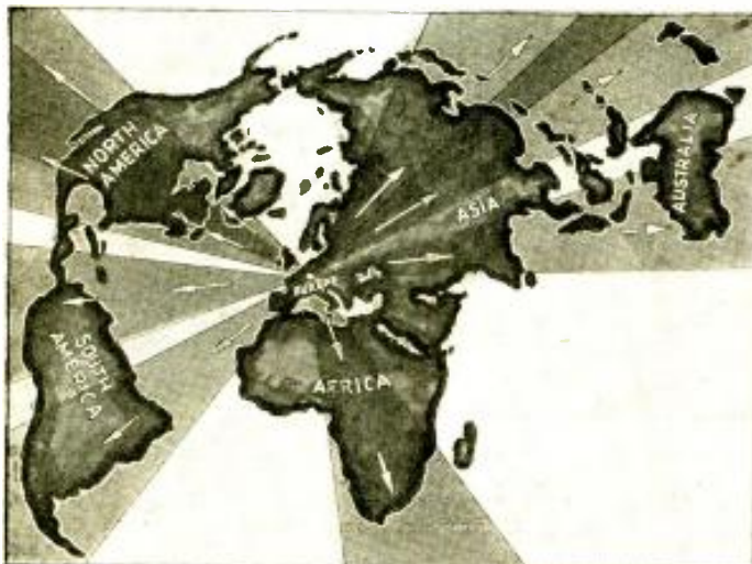
The shaded areas of the map show the seven different beams employed by the German short-wave station when broadcasting to different parts of the world.
