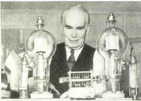
↑ Dr. Lee de Forest has turned his lifetime of experience to the building of radio therapy instruments. He has designed a machine known as the "Dy'natherm," which, by means of short waves, induces artificial fever, helpful in curing various ailments. Dr. de Forest is shown in his Los Angeles laboratory.
