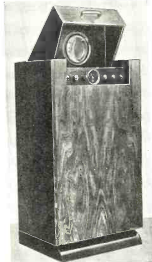
Fig. 4—The Radio L.L. television receiver, with vertical cathode-ray tube.
