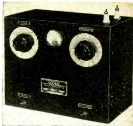
Front view of the 25-watt C.W. transmitter. No. 659
