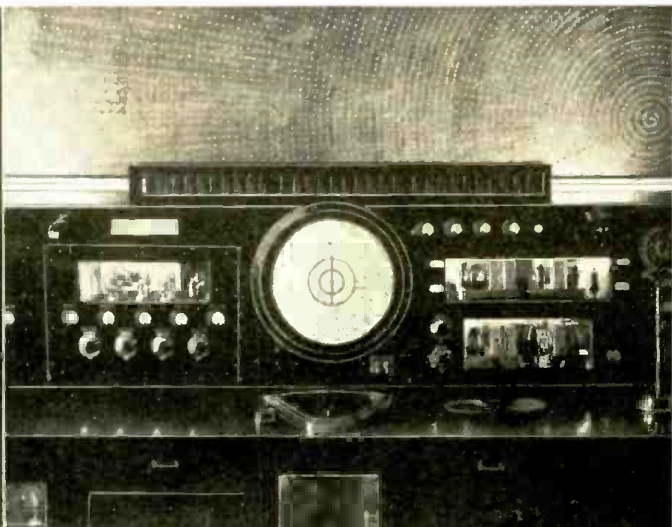
Photo at left shows radio control board for the Spitz Flight Recorder. The directional coils are seen mounted on top of the Binaural Selector, at the right of the picture. Landing map is seen in center of panel above the "divergence" wavemeter. Right hand photo shows panel-board with map removed and the elaborate system of lights that progressively flash the plane's course behind the map.
