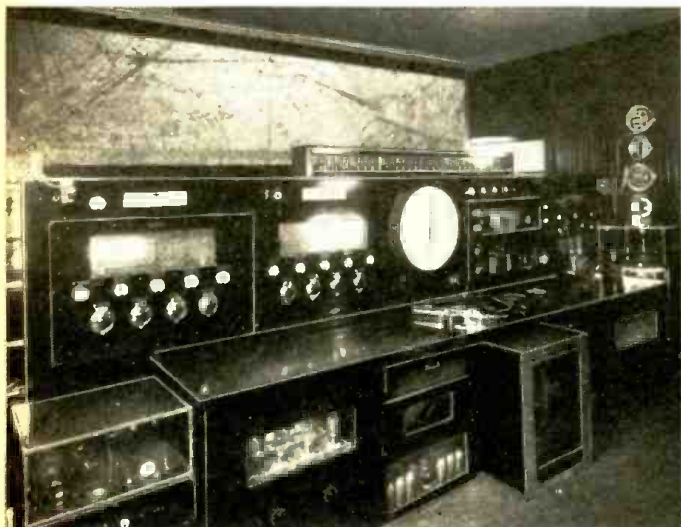
Photo at left shows radio control board for the Spitz Flight Recorder. The directional coils are seen mounted on top of the Binaural Selector, at the right of the picture. Landing map is seen in center of panel above the "divergence" wavemeter. Right hand photo shows panel-board with map removed and the elaborate system of lights that progressively flash the plane's course behind the map.
