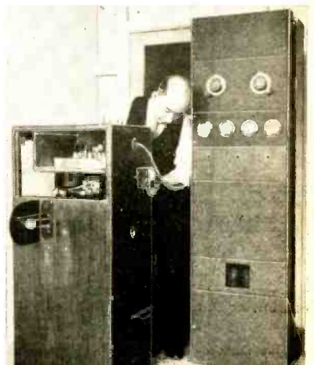
An engineer is shown in the act of checking the 6-volt exciter lamp on the transmitter. The short-wave transmitting panel is shown at the right of the photo.
