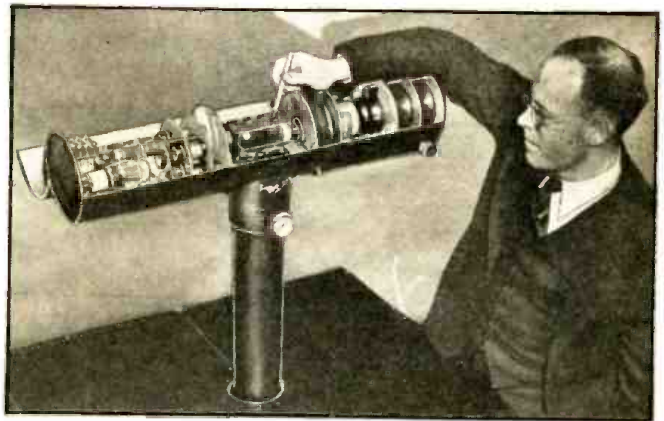
Dr. R. R. Law points to a newly developed "Electron Gun" in the new "Kinescope" for projecting Television images.
