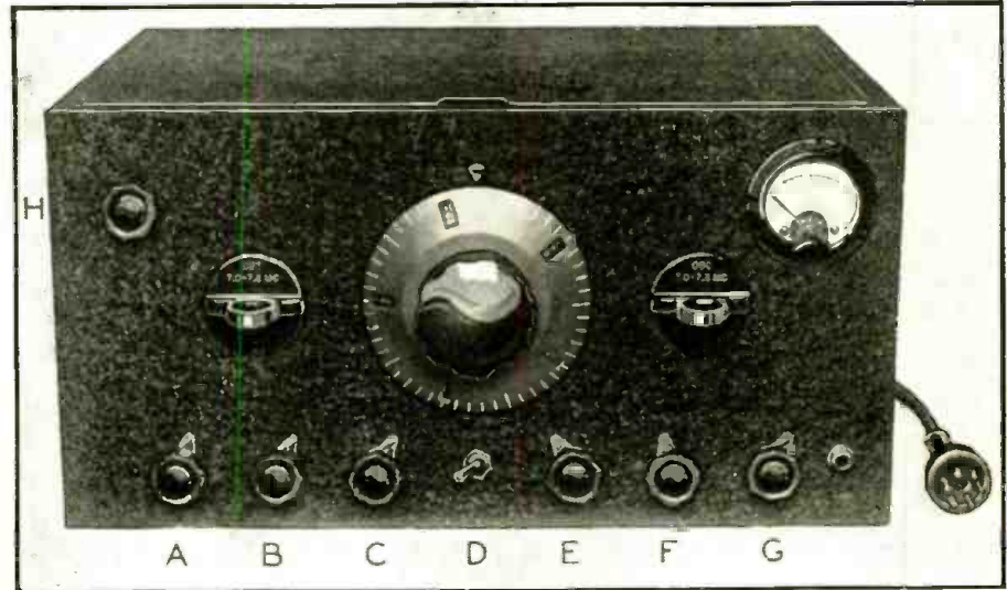
Front view of the receiver, the controls are as follows: A—First detector regeneration, B—Detector trimmer, C—R.F. gain and AVC switch, D—Beat oscillator switch, E—Noise silencer, F—A.F. volume control, G—Tone control, H—Crystal band-width control. The jack in the extreme right-hand corner is for ear-phone operation.
