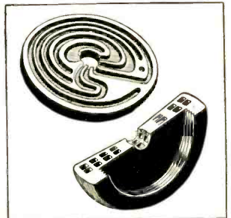
Cut-away views of the new high-quality earphone cap. No. 632
