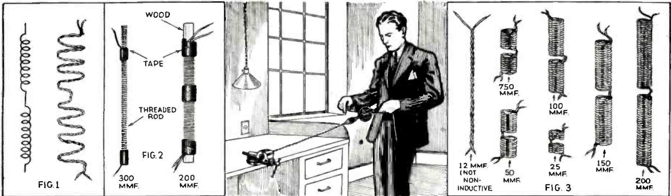
Various small capacities or condensers can be made up by winding insulated wire on to wood dowel sticks, fibre tubes, etc. By proper arrangement of the units, the condensers can be made non-inductive
