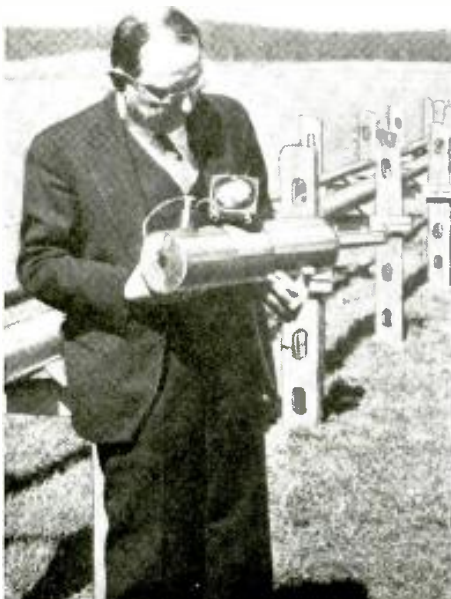
G. C. Southworth holding one of the resonant chambers used for tests of wave-guide transmission. Behind him are the two transmission lines.
