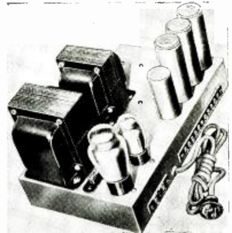
Physical appearance of the power supply unit which is built as a separate unit. It employs two rectifiers—a 5Z3 and a 1V.
