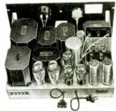
Right—rear view showing the extremely neat construction of the RCA 40-watt transmitter. (No. 524)
