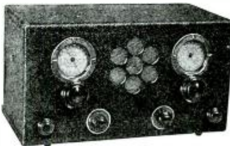
Sargent Model 10-5 Tube Receiver
