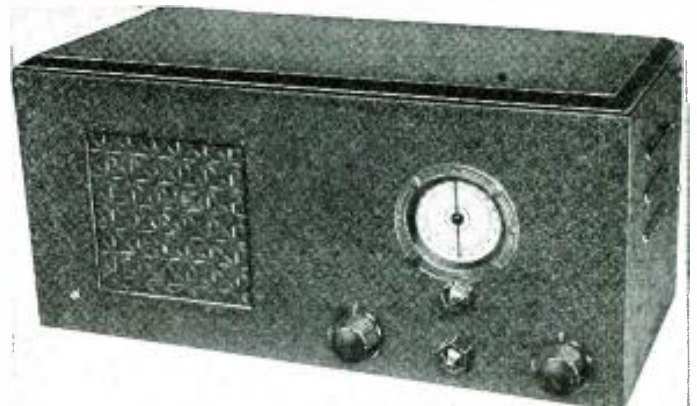
Note how the controls on this improved 5-tube TRF regenerative receiver have been compactly grouped at the right of the set.
