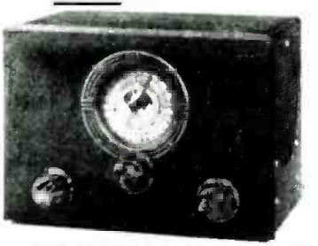
—1936 FULTONE V 3-Tube Receiver FIVE-IN-THREE • 6D6-6F7-12A7
