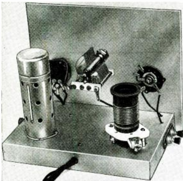
Rear view of the Regenerative Booster or R.F. amplifier.
