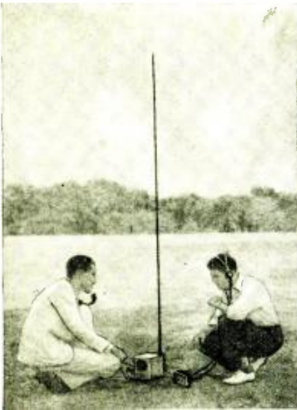
Photo at left—portable 5 and 10 meter combination "transmitter-receiver" in actual operation in the field. A telescopic antenna is very desirable for the purpose. Plate and filament supply is readily obtained from batteries.
