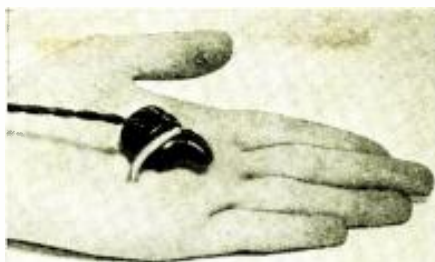
Here is the very latest style earphone for radio receivers—it weighs but 2 ounces and fits right into the ear. It has a resistance of 2000 ohms. (Refer to No. 118.)
