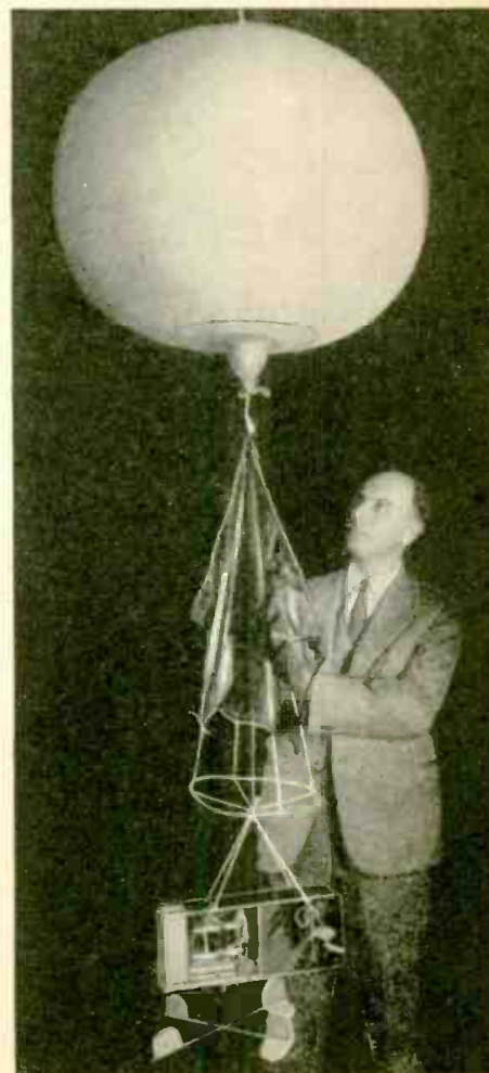
We recently described a European S-W transmitter sent up, attached to a balloon, for signaling the upper air conditions to weather observers. This photo shows similar apparatus used by the U. S. Weather Bureau.
