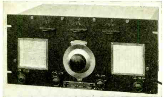
Front view of new "AGS" commercial or "pro" type short wave receiver, with "single dial" control. Yes, it's a super-het!
