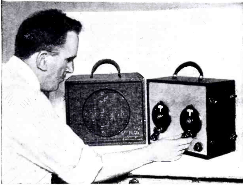
H. W. Secor is here shown trying out the 8-Tube Portable "All-Wave" Superhet designed by Mr. Denton.
