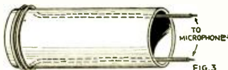
Absorption-modulation coil wound on a tube; the terminals connect to the microphone.
