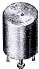
Hammarlund Shielded Polarized Choke. High inductance, low distributed capacity.
