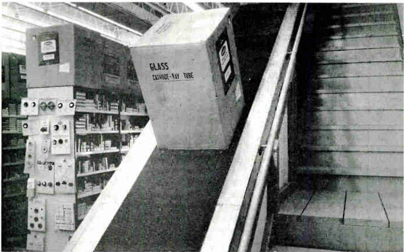
The conveyor system enters the main floor from the ceiling next to the stairway. There is a similar unit going to and from the basement. The stairway and conveyor system take up only six feet of floor space. The second story is used entirely for the storage of new picture tubes and the basement for other items. A third conveyor from the outside permits unloading of stock at a minimum of man power.
