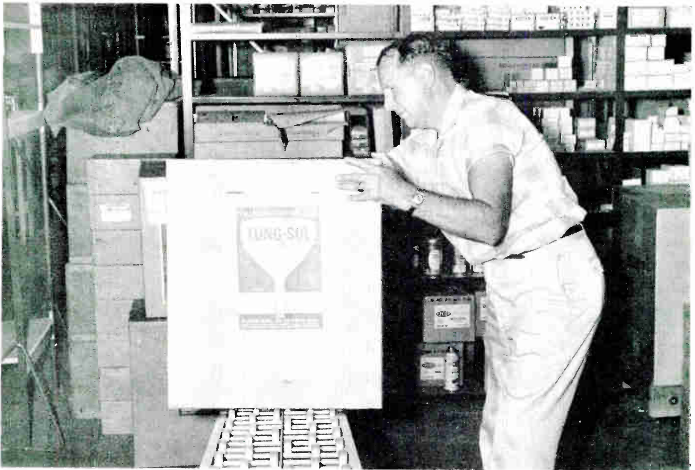
Roller conveyor frames for unloading fragile and bulky picture tubes.
