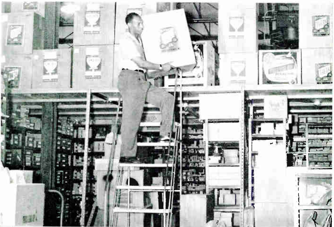
Picture tube storage utilizing metal framing elements. Note safety ladder.
