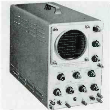
Scope (in kit form) featuring dc coupled amplifiers and CR tube unblanking. A 5ADP2 flat face CR tube is used for accurate readings on an edge-lighted grid screen. A conetic-fernetic CR tube shield prevents trace distortion by stray ac fields. (OP-1; Heath Co., Benton Harbor 11, Mich.)
