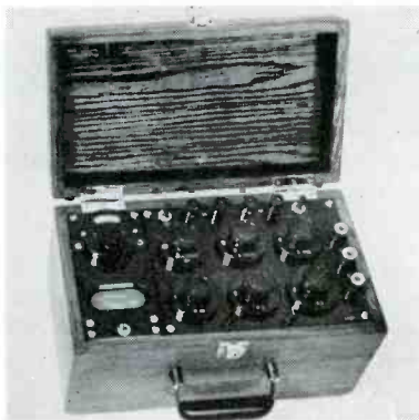
Portable Wheatstone bridge which measures resistors from 100,000 ohms to 1.5 megohms to an accuracy of .1% and up to 10 megohms to an accuracy of .25%. (1071; Minneapolis-Honeywell Regulator Co., Rubicon Instruments Div., Ridge Ave. and 35th St., Philadelphia 32, Pa.)
