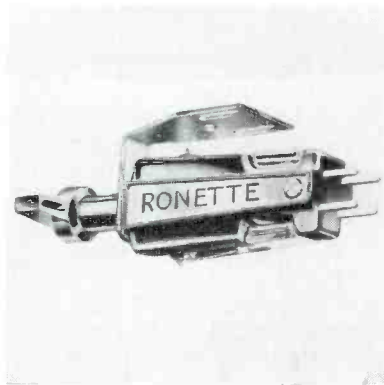
Four-terminal dual-element cartridge with recommended tracking pressure of 4 to 6 grams. Frequency response is said to be flat from 20 to 15,000 cycles with a roll-off at 14,000 cycles. (Binofluid; Ronette Acoustical Corp., 190 Earle Ave., Lynbrook, N. Y.)
