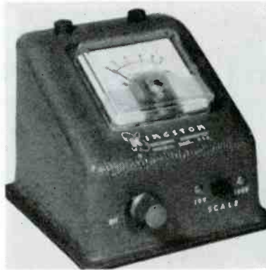
Battery-driven variable dc power source covering the range from 0 to 67.5 v. Unit produces negative bias voltages for agc troubleshooting, alignment and experimental or laboratory work. Features a two-scale meter for accurate setting and correcting for various load conditions. (BB-1; Kingston Electronic Corp., Medfield, Mass.)
