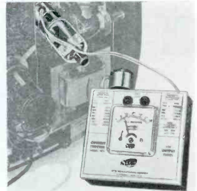
Current checker for horizontal output circuits which can be placed in circuit without disconnecting cathode. Indicates whether cathode current of horizontal output deflection tubes is within manufacturer's recommended limits. (HC-6; Seco Manufacturing Co., 5015 Penn Ave. S., Minneapolis, Minn.)
