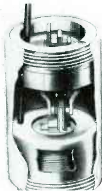
VIBRATOR (interruptor, full wave for 6 or 24 v) that is only 1/4" long, 3/4" in diameter and weighs 1 1/2 ounces. Primarily designed for short cycle use only. Maximum performance is obtainable under such cycles as 5 to 20 minutes on and 1/2 to 1 hour off. The vibrator was engineered for applications such as beacons, airborne equipment and other uses where extremely small size and light weight are important factors. (P. R. Mallory and Co., Inc., Indianapolis 6, Ind.)
