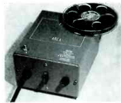
HEAVY-DUTY degausser to erase magnetic tape without the necessity of re-winding. Degaussing removes residual magnetism present on tape as a result of recorded impressions or random magnetism that sometimes occurs during storage. Demagnetization is accomplished by placing tape over spindle provided, and rotating the reel three or four times until every portion of the tape has been exposed to the field area which exists within the rectangle outlined on the top of the degausser. Continuing rotation, the reel is slowly lifted off the spindle to height of approximately 6" to 8" and power is then turned off. (Model 710; Aerovox.)
