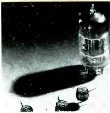
FIG. 2: NEWEST TYPES of transistors available for electronic control and computing equipment. Transistor below, a power tetrode (Minneapolis-Honeywell), can be used to operate on a 28-volt system with currents up to 10 amperes.
