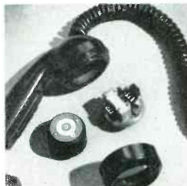
(Left) TRANSDUCTANCE-TYPE MICROPHONE that includes a two-stage transistorized amplifier built into the same capsule as the microphone unit. Microphone was designed to replace the older carbon button types.
