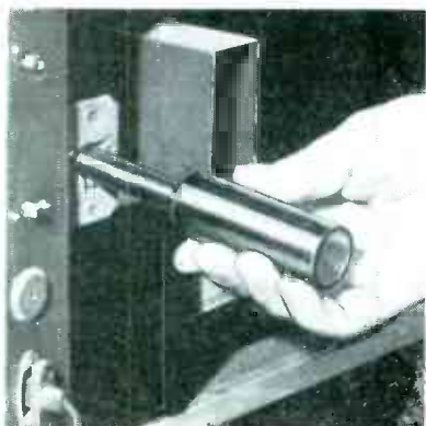
ABOVE: COLOR-TV cheater , an installation-service safety device. This tool permits use of a high-voltage probe and allows the set to operate with the back removed.
