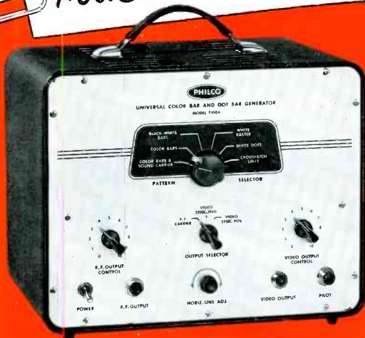
PHILCO 7100A—Newest Philco Universal Color and Dot Bar Generator
