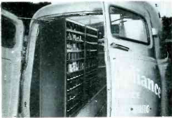
PANEL TRUCK of a service shop, used for field installation and repair, equipped with a storage unit with a combination of drawers and bins which can hold tools, hardware, components, test equipment, tubes and accessories. (Equipto)
