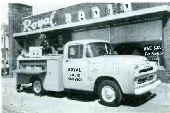
PICKUP TRUCK fitted with side-compartment type utility body which can not only be used to store tools, parts and accessories, but chassis going to or from service shop. Installation equipment which can be carried on trucks of this type include overhead rack with adjustable ladder, side-mounted brackets for pipe or conduit and adjustable mounting bracket for pipe threader. (Dodge Trucks)
