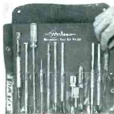
ABOVE: KIT OF ALIGNMENT and specialty tools , which includes solder-erase and wire-dressing tools, alignment screw drivers, stubby-stud drivers, double-ended hex aligners and a pocket container of lubricating oil. (Walsco.)
