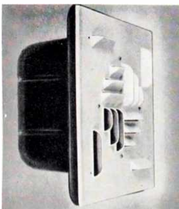
BASS REFLEX ENCLOSURE said to replace one standard acoustical tile when used in ceiling installations. Unit consists of a plaster ring, bass reflex enclosure and spiral sound faceplate which incorporates directional ports to provide a 360° dispersion pattern. Present model accommodates 8" speaker. (SBR 8 DS; Fourjay Industries, 2360 West Dorothy Lane, Dayton 9, Ohio.)
