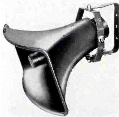
ALL-WEATHER wide-angle (30 w cont; 50 w peak) pa speaker with an acousti-matched built-in driver (reproducer) unit. Has a one-piece main flare and unit cover; a pressure moulding of reinforced polyester fibreglass. (Model CP-44 King Cobra-Jector; Atlas Sound Corp., 1451 39 St., Brooklyn 18, N. Y.)
