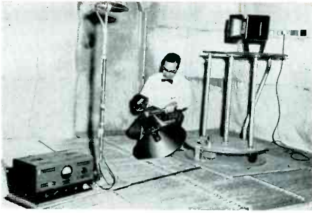
ABE COHEN , engineering manager for University, applying a driver unit into a reflex trumpet preparatory to testing for polar-frequency response. Wide-angle trumpet, on stand, has just been similarly tested.
