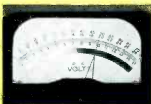
Low “fixed bias” point at -1 volt (bottom scale)
