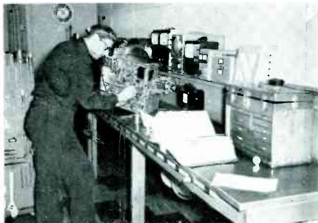
TV REPAIR bench at BDM. Tool rack, at left, is mounted on a dolly for mobility. All tools are held in place by friction clips.
