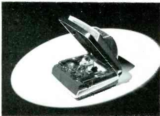
ABOVE: TRANSISTOR RADIO in its plastic cabinet with speaker in hinged cover. Top view of complete chassis is at right.
