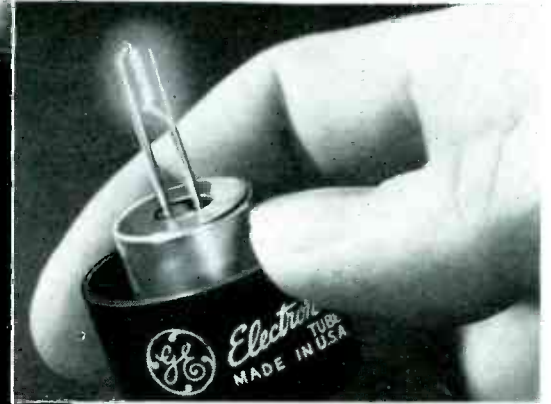
ABOVE: Tungsten "lightning rod" in G-E high-voltage rectifier tubes shields the filament from electrostatic pull of high anode voltages. Shorts, broken filaments are sharply reduced.
