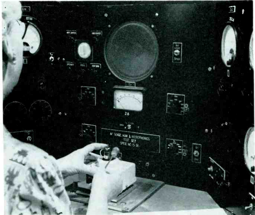
LAB TEST set operator testing a 12AX7 miniature twin triode for af noise, microphonics and hum. With this test, spurious signals generated by automatic or hand tapping, and hum originating within tube, can be measured for amplitude by output meter, and analyzed by ear with speaker.
